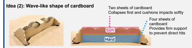
By making the ends of two of the four sheets of corrugated cardboard layers wavy and overlapping them in an alternating pattern, TOTO has also made it easier to collapse the layers intentionally. This enables the ends of the two sheets to which the impact is applied to receive the product softly, and then all four overlapping layers to firmly cushion the packaged item.
